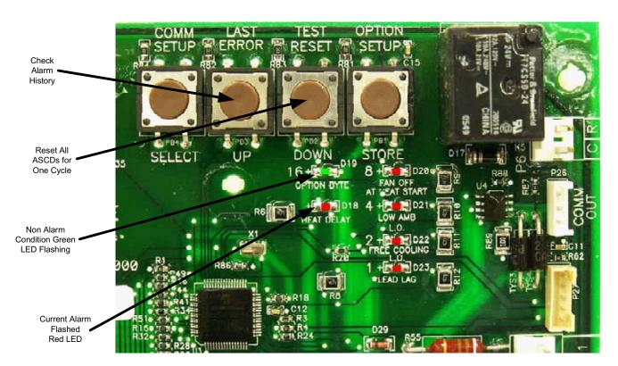
FIGURE 24 - UNIT CONTROL BOARD
